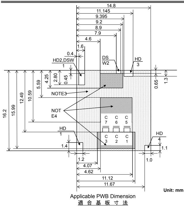
NOTE3. ONLY GND PATERN AND GND VIA HOLE IN ALLOWED IN THIS AREA. NOTE4. NO PATTERN, VIA HOLE IN THIS AREA.
